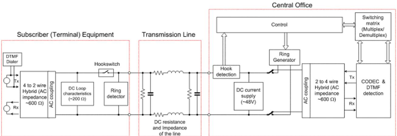
The telephone company applies loop feed DC voltage between Tip and Ring at the Central Office (CO). This voltage is 50 Vdc on average. Terminal equipment should be able to operate with both positive and negative voltage polarity.
