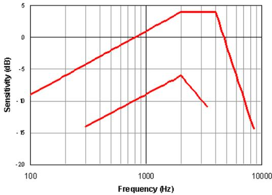
Figure 4. TBR 38 Receiving Sensitivity Limits.
